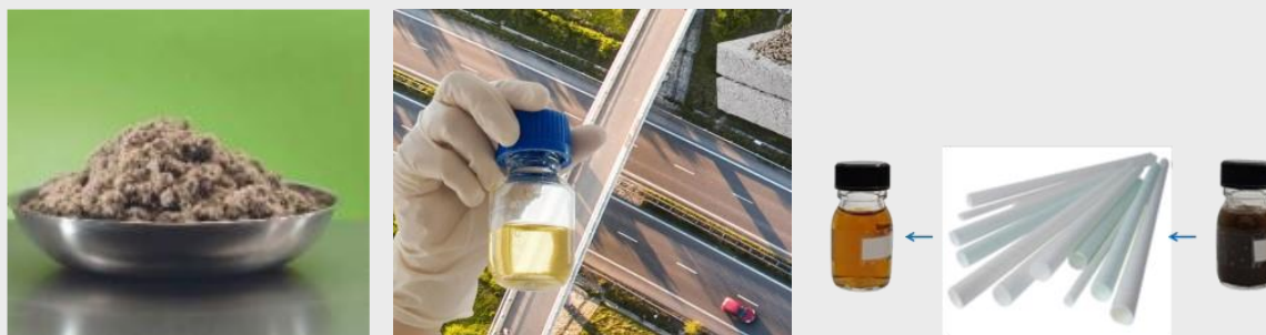
Renewable third generation cellulose (left) and glucose (middle) obtained from residual streams, hydrolysate before and permeate after membrane filtration (right)
