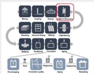
Schematic LIB manufacturing process
