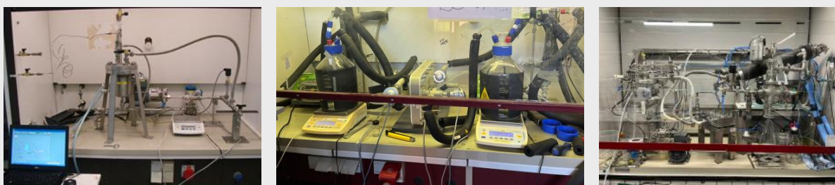
Figure 2. Small bench-top unit (1 L) for membrane filtration screening (left), membrane distillation unit (middle), and pervaporation unit (right)
