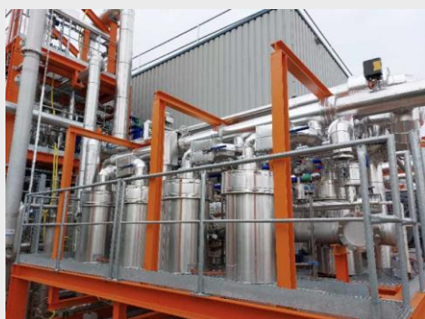
Hybrid distillation-pervaporation for IPA dehydration (left) and Pervatech pervaporation pilot (right)
