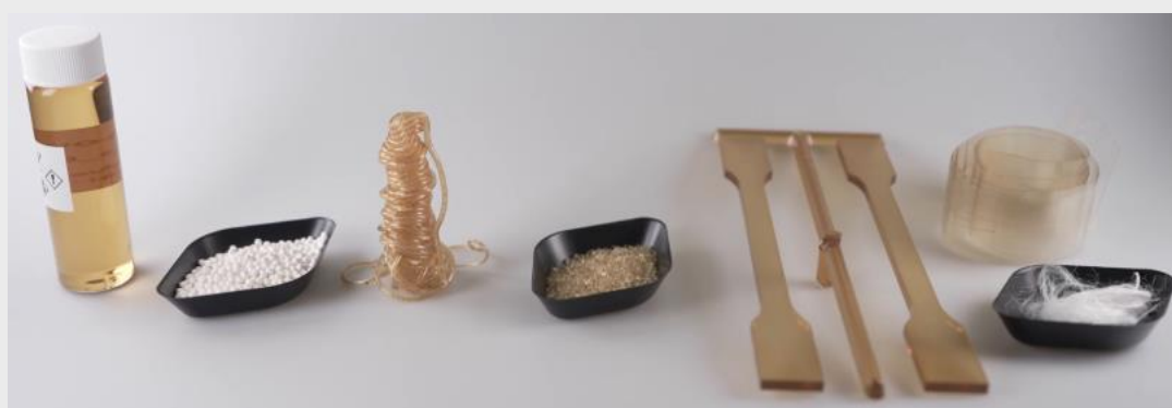
Figure 1 Different processing forms of PRIOLON, from polymer solution to extruded materials.
